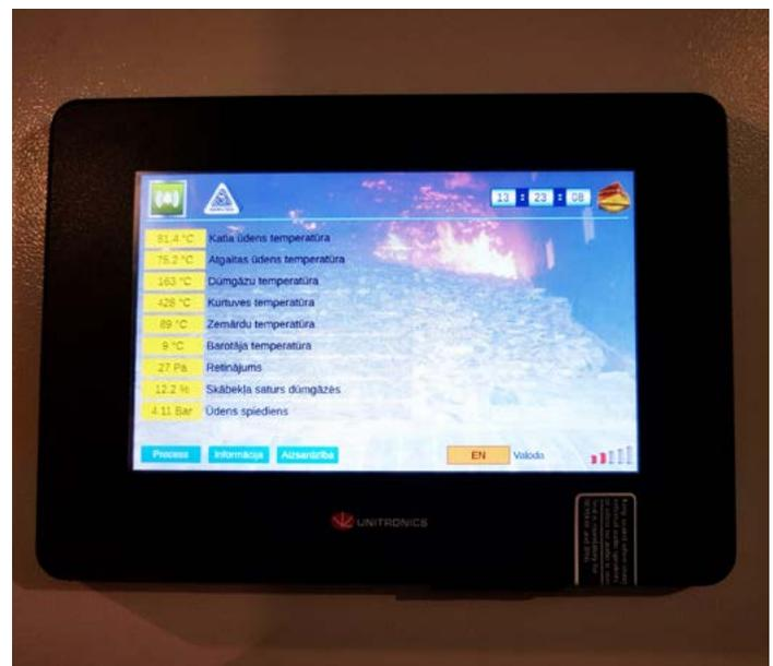
(text message). Remote control is provided via modem communication. The boiler room has video surveillance, as well as fire and security alarm systems. Thanks to the integrated data processing system from the connected IP cameras, the controller displays the video (stream) in real time and is able to play the sound.
